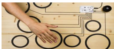
Figure 4. An example of wooden interfaces to the Video Projection Tool.
