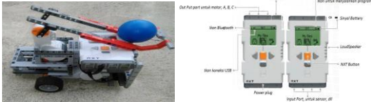
Figure 1: The completed LEGO Mindstorms NXT 2.0 (8547) and NXT programmable intelligent brick
