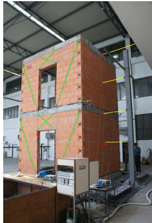
Figure 4. Typical test model of building
